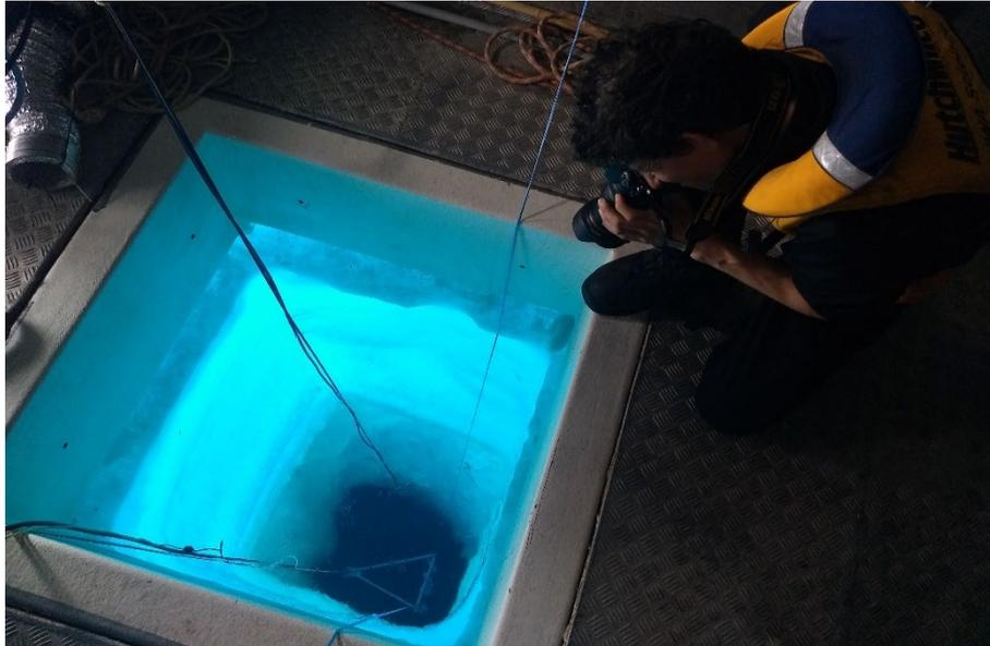
*Brett Grant (NIWA) photographs the sea ice, platelet layer and window to the ocean through the hole in the base of the converted shipping container. The blue colour is sunlight which has made its way into the ocean, filtered through snow, sea ice and platelet layers. (Image credit: Natalie Robinson)*
